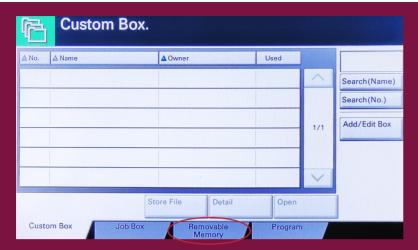
• Press the **Home** button on the physical keyboard of the device and then select the **Removable Memory** icon on the screen:
